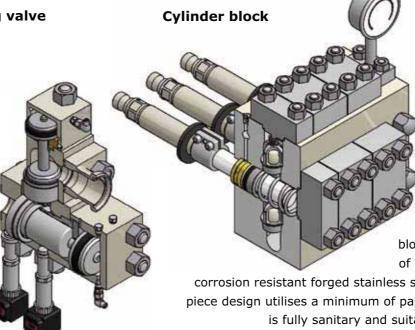
The pump block is a one piece precision machined block, made out of high strength
